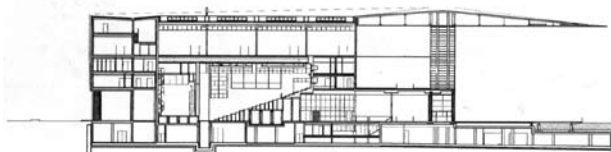
longitudinal section through Middle Hall
