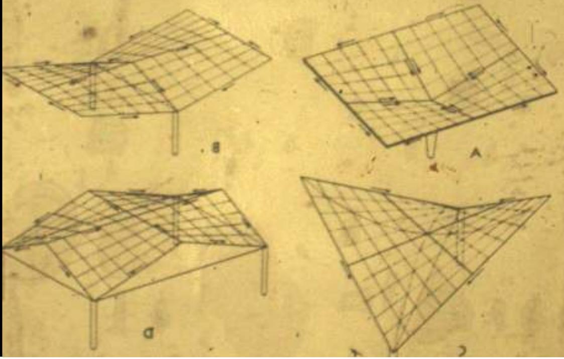
Figure 13 Derivation of a hyperbolic paraboloid
